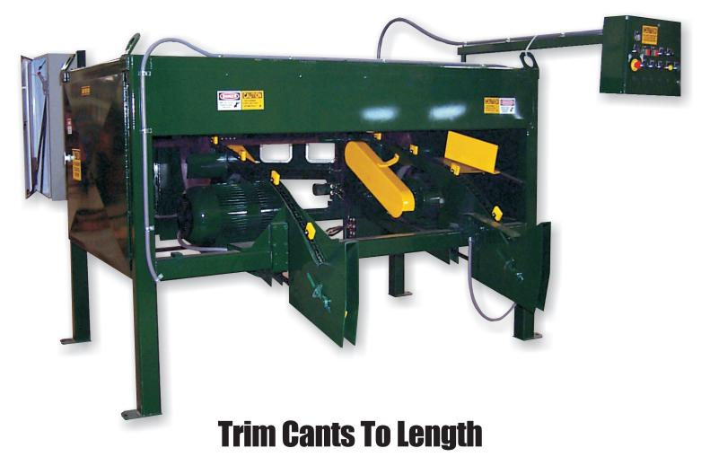
Originally designed and manufactured to work inline with our 6800 and 6900 Scragg Mills, the Pendu 6600 tow headed trim saw is the easy, efficient way to cut cants to length. Dual saw heads, one stationary and one adjustable, driven by powerful 15 HP electric motors power through material up to 6" (10" Opt.) in depth. The adjustable head will cut cants from 28" up to 72" (120" Opt.) in Length.
