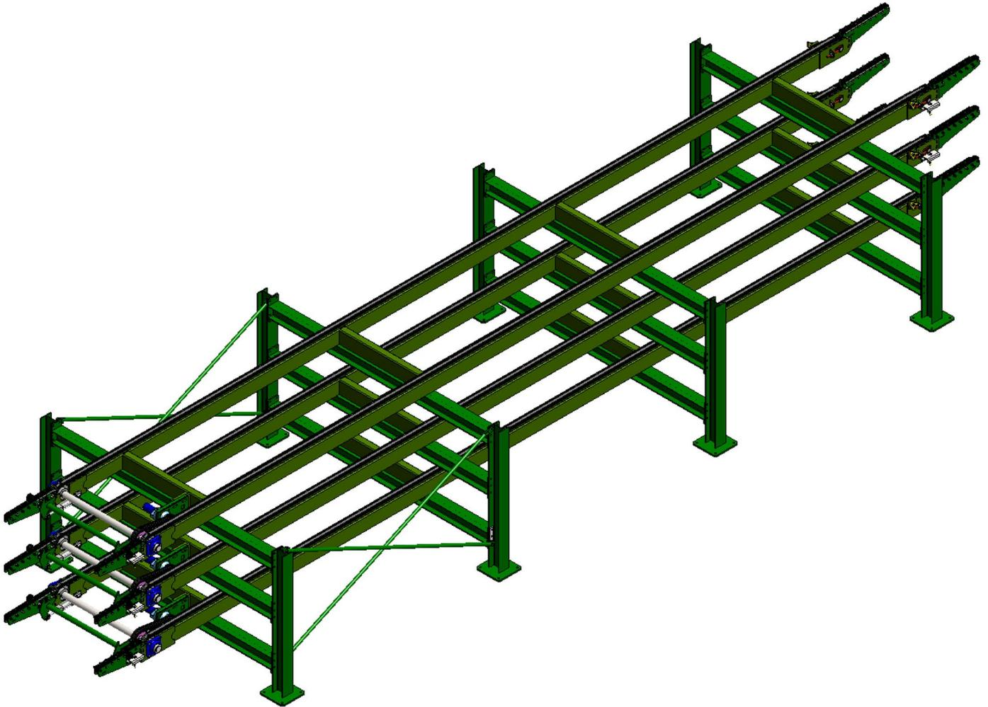
Pendu Railway Tie Sorting Decks collect ties from your production line and sorts them onto multiple levels. 35' long accumulator chains hold approximately 77 ties at a time.
