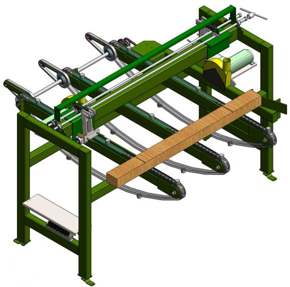
The Pendu Tie Kerf Saw makes an accurate kerf for perfect track line side alignment. Two saw blades make a 3/16" kerf. The machine is powered by 5 HP electric motors.
