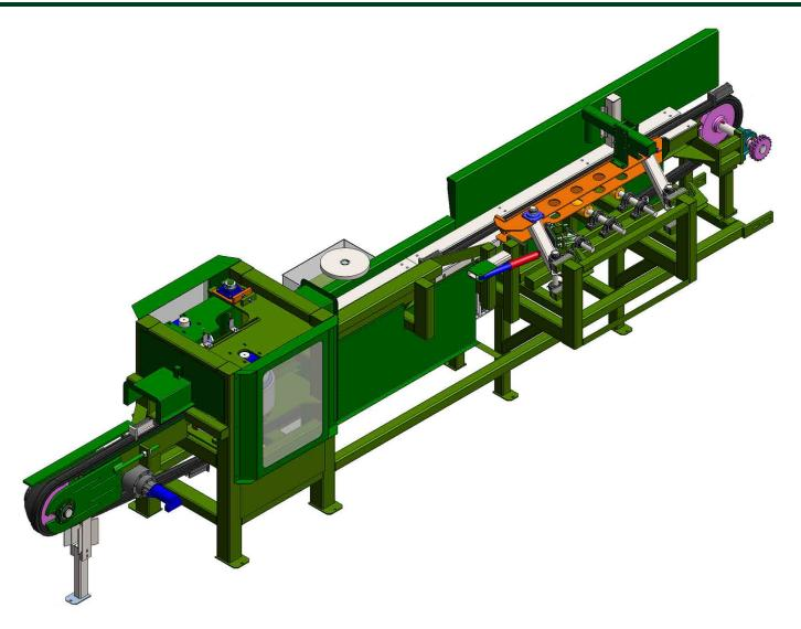
The Pendu Incisor features a Hydraulic driven lugged chain to push each tie in order to get a full length incise from end to endwhich runs at 10 lugs per minute. Hydraulic cylinders actuate the incisor drums. Material can be either 6' x 8' or 7' x 9'. The Railway Tie Incisor will produce crossties up to 9' long.
