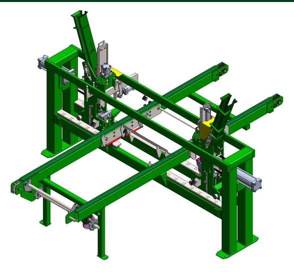
The Pendu Crosstie Plater is capable of applying plates to both ends of ties at a rate of ten ties per minute. The end plater automatically deals a tie, finds the ends (6' 6" – 9' range), squeezes any cracks out of ends (15,000 lbs each direction), issues plates (either 5" x 6" or 6" x 7"), and presses them on each end (70,000 lbs). The manually loaded magazine has a 36" capacity.
