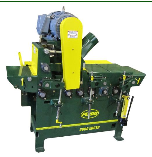
The 3000E single arbor gang saw is designed to handle your MRR & S4S lumber up to 2 1/2 inches in thickness and up to 24 inches wide. The 3000E will rip through boards quickly allowing you to increase your production. The machine can be equipped with the optional top sizer head for sizing material for thickness (top sizer head shown in above photo). The 3000E can be set up to run fixed width and random width material.
