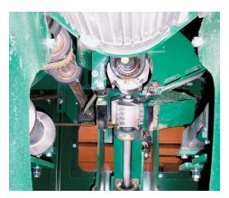
pass through a series of computer-controlled cutter-heads that randomly engage the surface at different depths and widths, simulating the finish of true hand-hewed logs.
