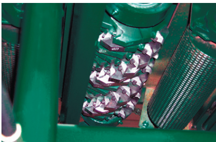
12" wide planer head with carbide insert can remove up to 1" from the sides of cants.
