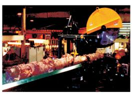
with a hydraulic driven 12" log chain. Also included are holding clamps that are spring loaded and console controlled and an outfeed log conveyor. If you need a hard-working chop saw, the Model 1300 is built for you.
