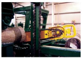
with a hydraulic driven 12" log chain. Also included are holding clamps that are spring loaded and console controlled and an outfeed log conveyor. If you need a hard-working cutoff saw, the Model 1200 is built for you.
