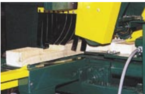
Fully adjustable cutter heads are mounted overhead for easier maintenance and set-up.
