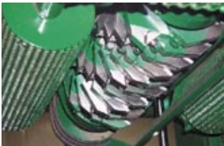
12" wide planer head with carbide insert can remove up to 1" from the top of cants.
